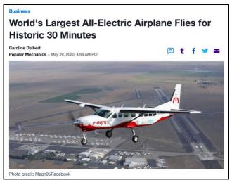
Electric, prop-driven aircraft are in certification trials to take over short-haul, low volume routes and specialty flights, and European manufacturer AirBus has begun work on a liquid hydrogen-fueled fanjet but currently, all hydrogen combustion comes with NOx emissions.
