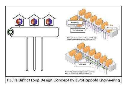
HEET, BuroHappold, Eversource, and various consultants finalized a pilot proposal to convert several "neighborhoods" within the gas system. Regulators were approached, and a pilot plan was approved. After underground thermal conductivity was tested in the fall of 2022, Eversource Gas broke ground on the geo micro-district in May, 2023. However, the unique nature of this work goes beyond the substitution of geo for gas.
