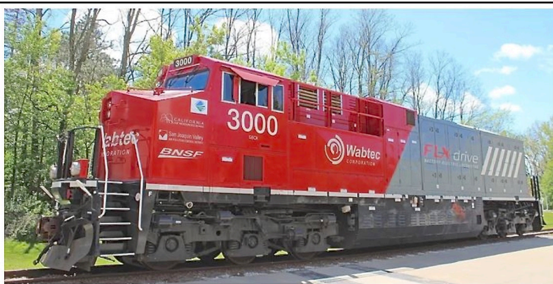
BNSF Railway and Wabtec pilot-tested a battery-electric locomotive in California in 2021. (Wabtec)
